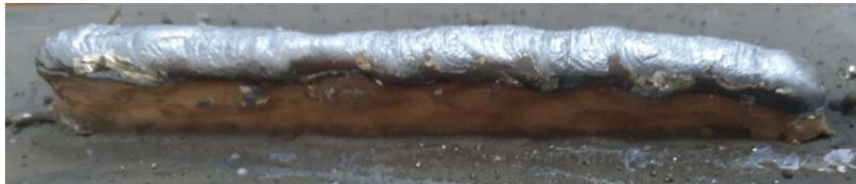
Figure 5: Slope at the end of the wall
