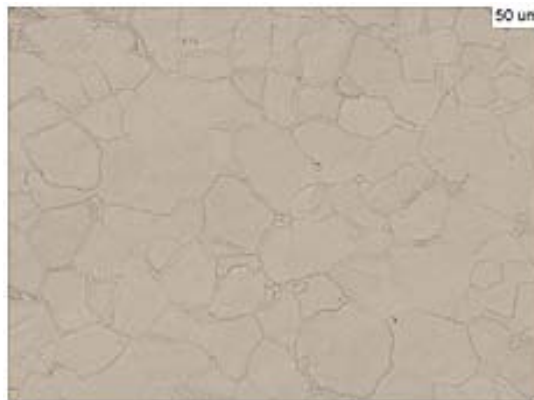
Figure 13: The microstructure of the middle sector (ferrite)
