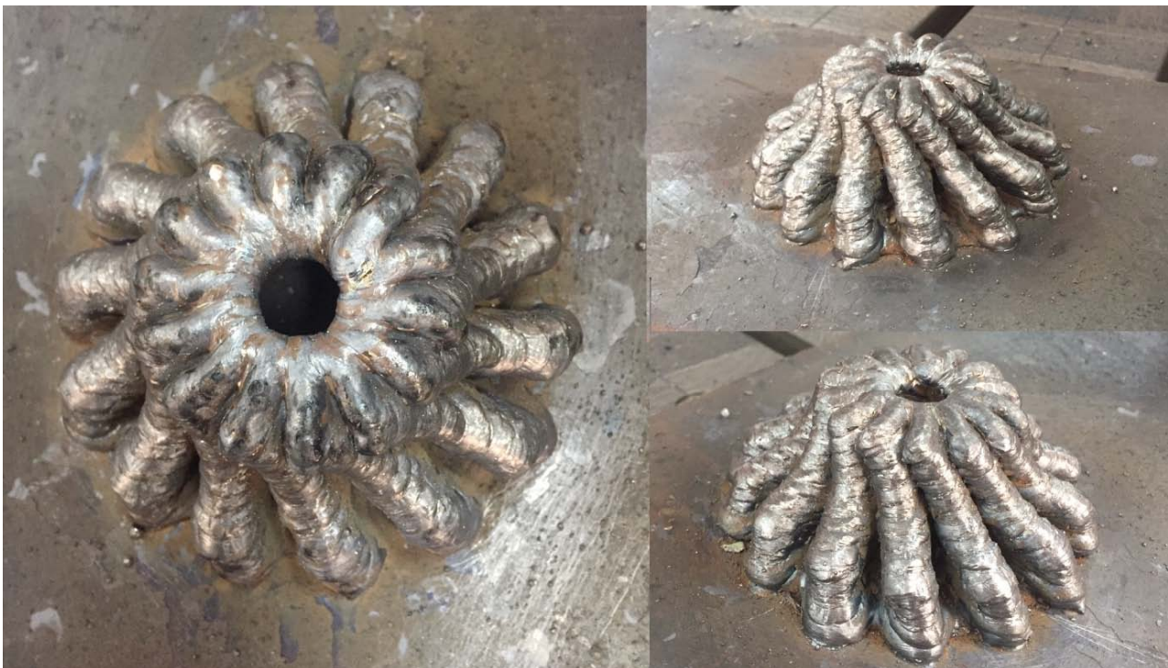
Figure 9: Compressor impeller prototype
