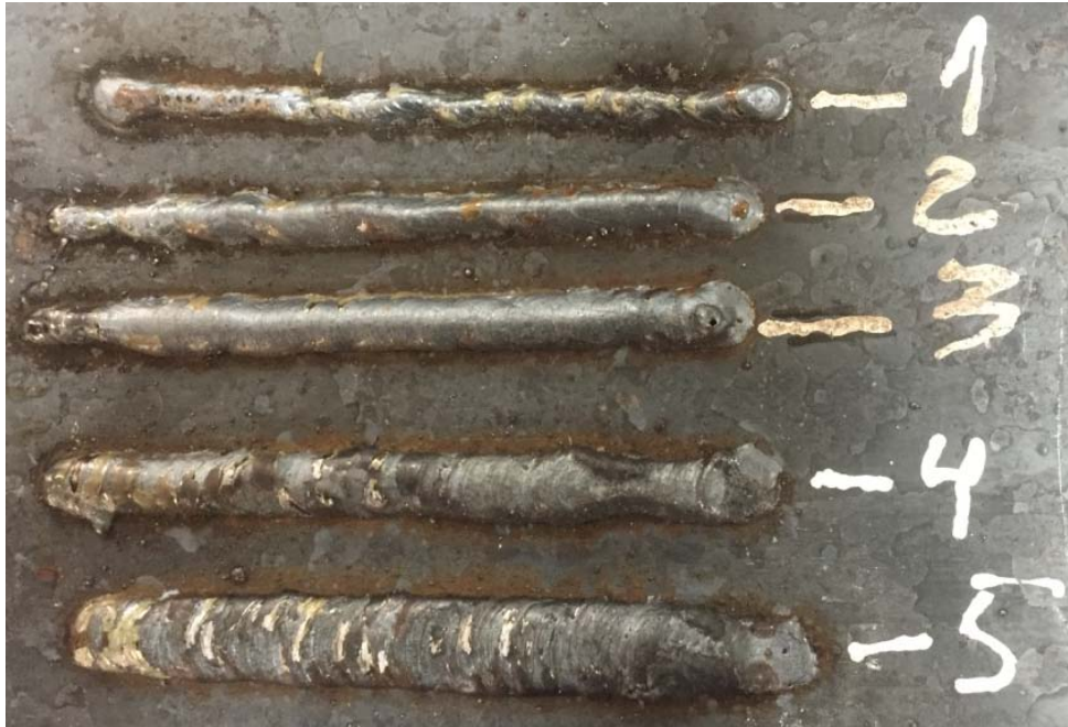
Figure 2: Deposited beads using different process parameters
