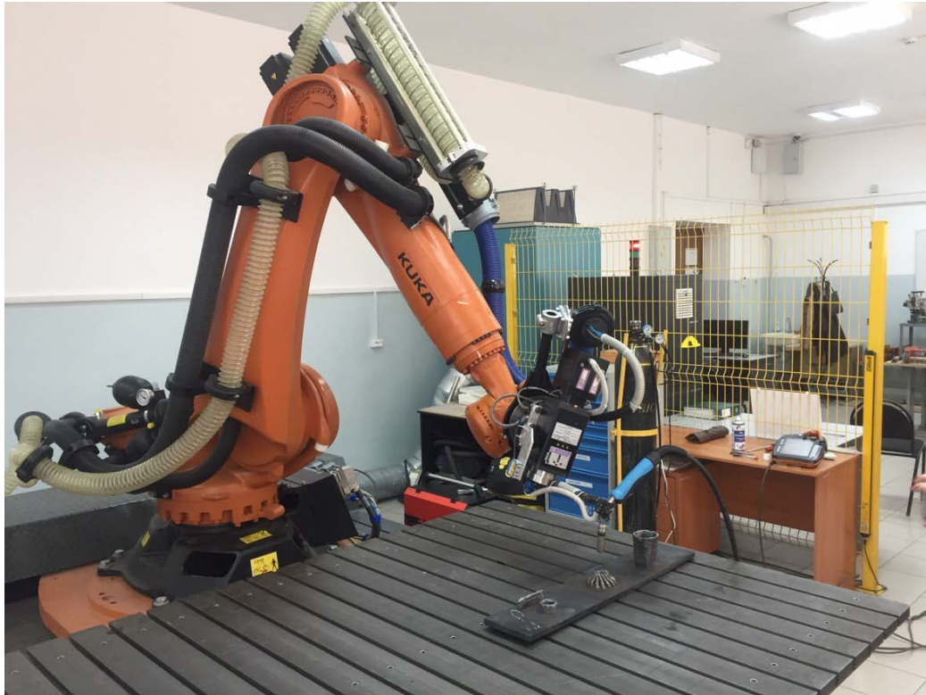
Figure 1: Experimental robotic WAAM complex
