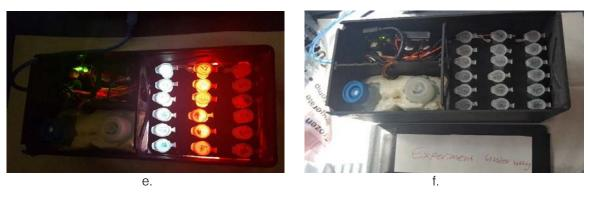
Figure 2: Preparation of samples at the PPF. a. Integration of Payload at Payload Processing Facility (PPF). b. Samples kept in the electric heater at PPF. c. Placing tubes with Spirulina in the NanoLab. d. Two sets of 18 tubes with Spirulina or flight and control. e. NanoLab housing the Spirulina flight samples. f. NanoLab housing the Spirulina control samples.
