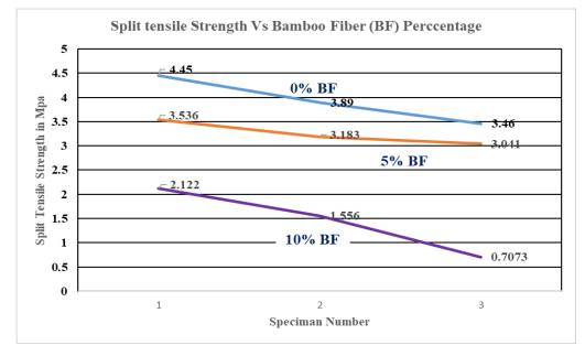
Steel fibers up to 1.5% with aspect ratio around 60 provide excellent TS to geopolymer concrete [6][10][13]. But with bamboo fibers up to 10% the relation between CS & TS in GPC is seriously affected with the coefficient varying from 0.3 to 0.75. The alternate way to use BF is to partially use steel fibers along with BF so that the loss of TS is brought back into material by steel fibers. This needs further research on this.
