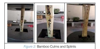
The splint without node have taken load 24.65 kN with 131.2 Mpa as tensile strength (average) while that with node developed 127.8 Mpa as average tensile strength. As seen in the figure 3, the failure of splints followed linearity up to yield points. The splints with node show three different slopes while without node
