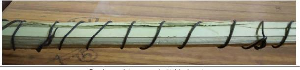
Bamboo splints wrapped with binding wire
