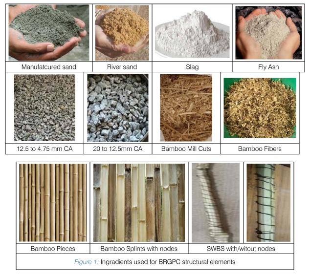
*Manufactured Sand:* Angular & rough texture need more water. Moisture is not held. Develops more strength compared to river sand. Silt content is zero. Granite compressive strength 100 to 250 Mpa and E = 20 to 70 GPa. M-Sand, crushed from granite stone, having Sp.gr 2.45, Fineness Modulus (F.M) 2.70.
