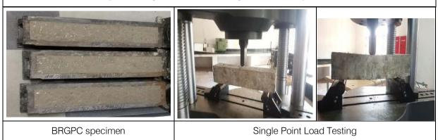
Figure 5: One point load testing of BRGPC sections
