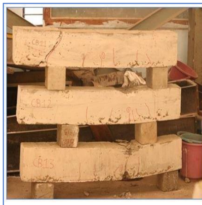
Fig. 10: For conventional beams of CB1 series, crack patterns with load deflection graph CB11, CB12, and CB13
