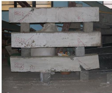
Fig. 12: Crack shape as well as Basalt-reinforced beams load-deflection graph
