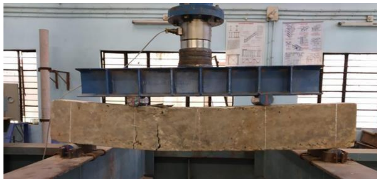
Fig. 4: Flexural Failure of beam
