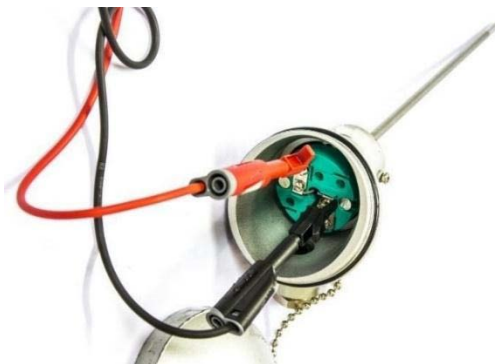
Figure 12: A Way to Calibrate an RTD
