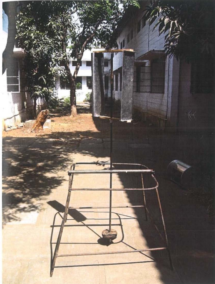
Figure 2.5: Experimental Setup With Giromill Rotor
