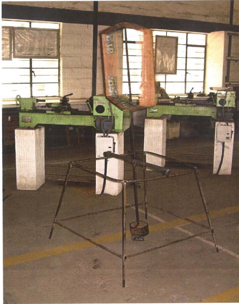
Figure 2.9: Experimental Setup With Simplified Darrieus Rotor
