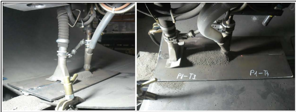
Figure 2: The Process of Submerged ARC Welding Samples in the Industry
