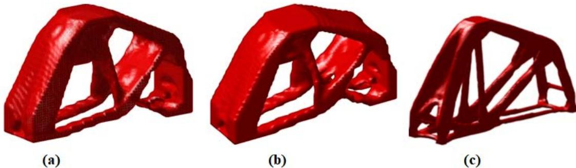
Fig. 6: Topology optimal for deep beam: (a) SESO-MMA; (b) SESO – OC and (c) VFSLM-MMA
