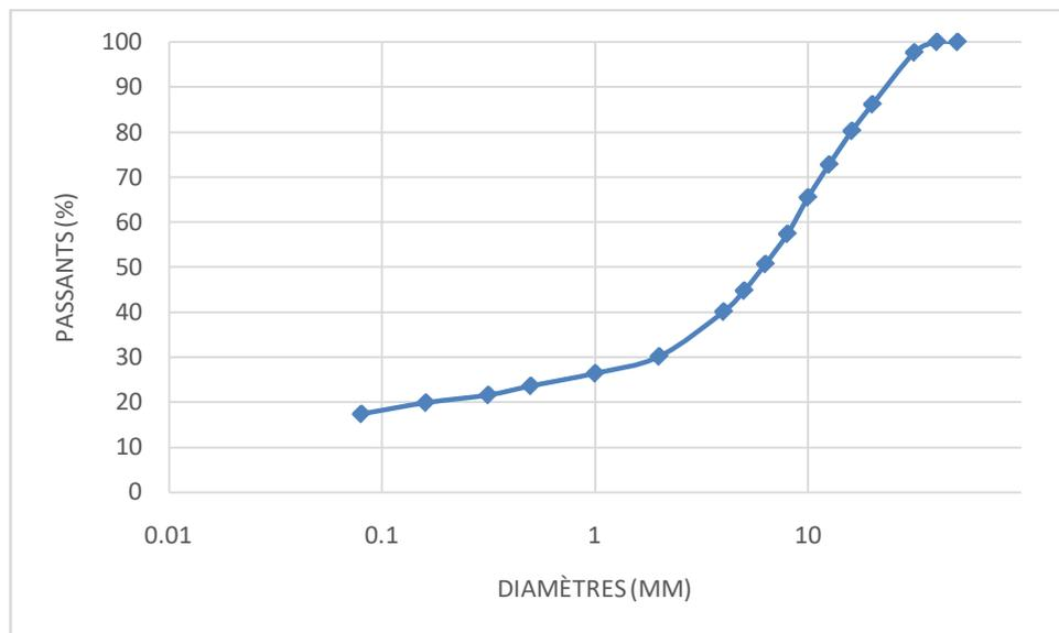
Figure 1: Particle size distribution curve of laterite
