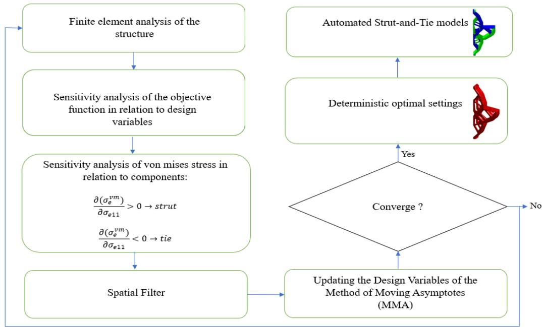
Fig. 4: Flowchart of the STM via TO
