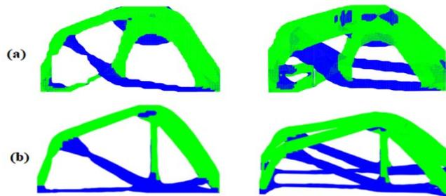
Fig. 8: Strut-and-tie models: (a) SESO; (b) VFLSM
