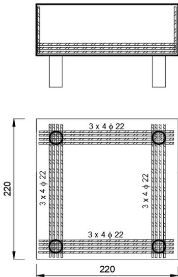
Fig. 12: Reinforcement arrangement for the pile cap
