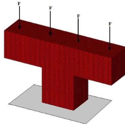
Fig. 13: Project domain of the Bridge pier
