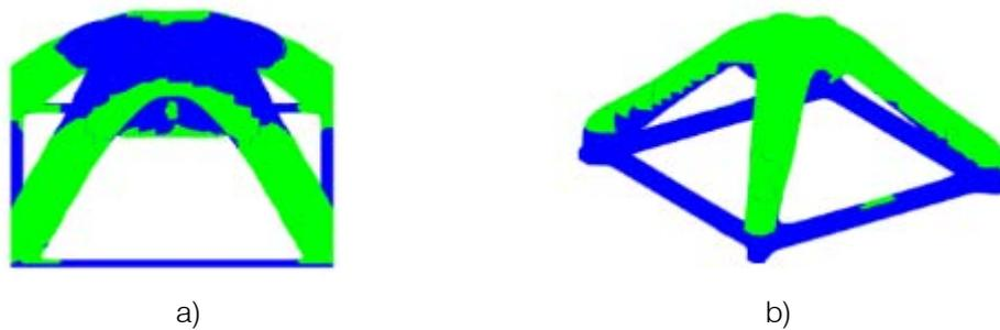
Fig. 10: Optimal topology: (a) SESO; (b) VFLSM (present formulation)
