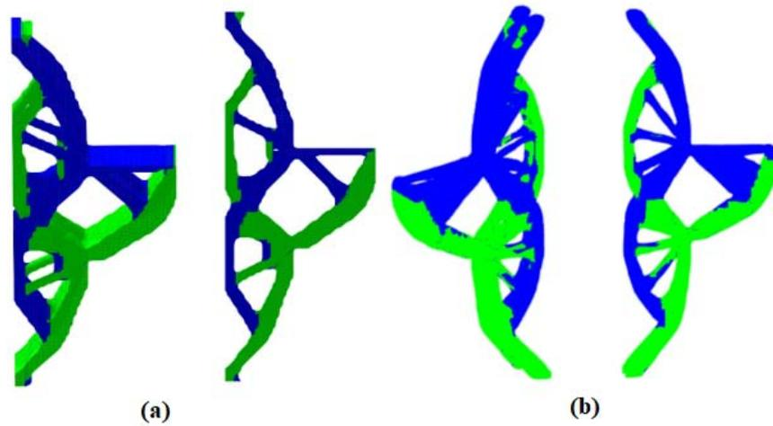
Fig. 24: Single Corbel, Strut-and-tie model: (a) SESO; (b) VFLSM
