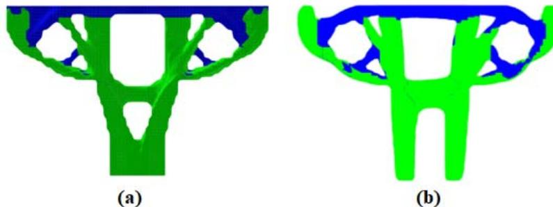
Fig. 19: Strut-and-tie model: (a) SESO and (b) VFLSM
