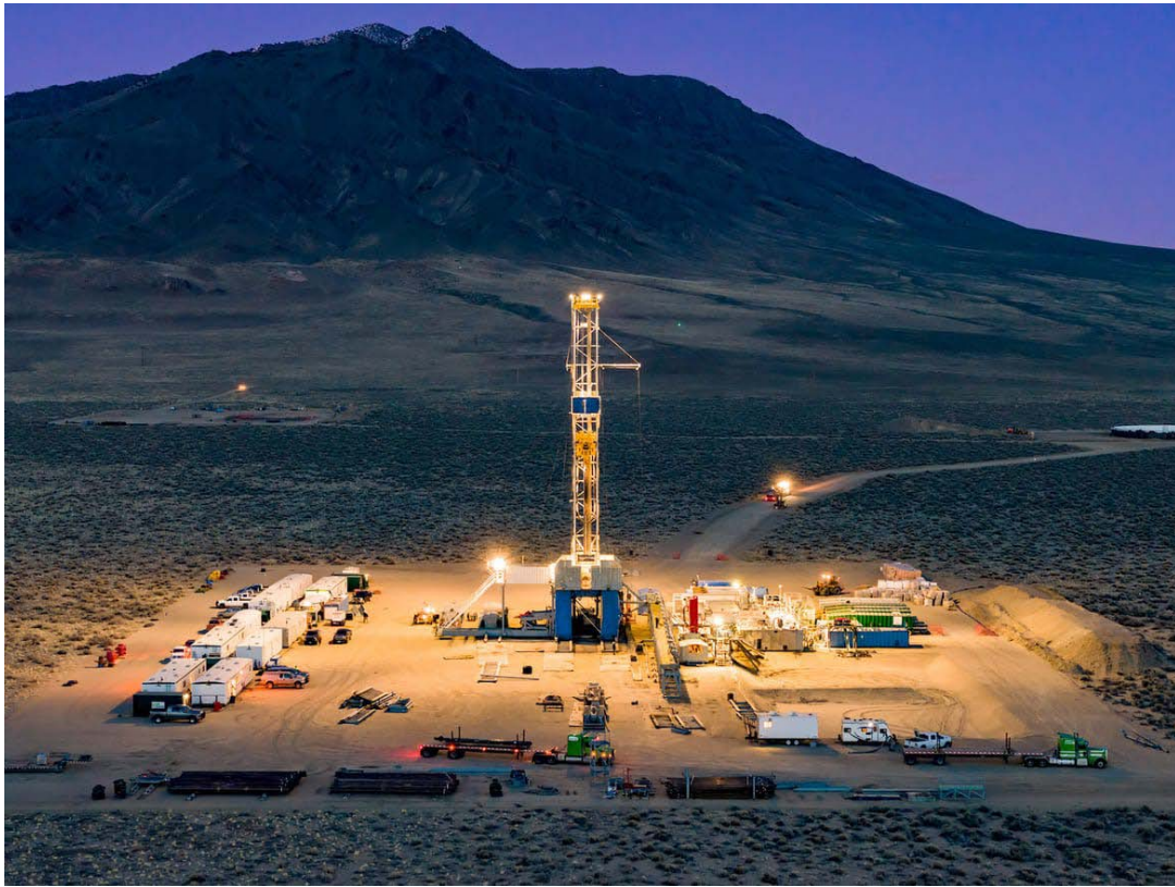
Fig. 4.5.2: Fervo uses horizontal drilling techniques to tap the earth's heat. Credits to Fervo Energy
