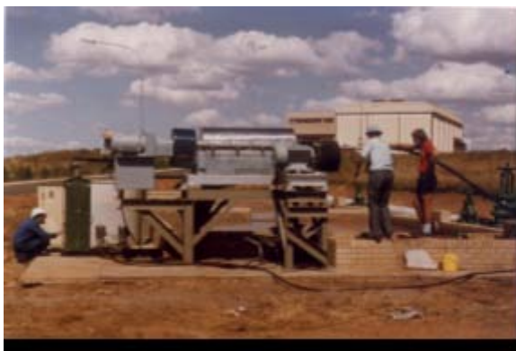
Figure 24: Sharples Polymizer 30000 centrifuge at the Saulspoort waterworks
