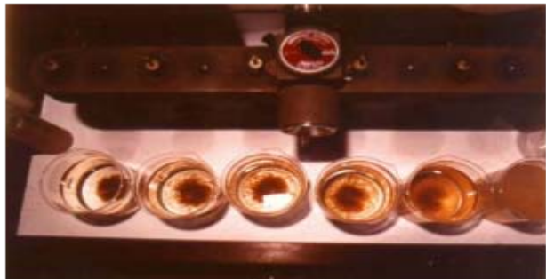
Figure 7: The effect of OAA dosing rate on settleability of agglomerates from right to left: NIL, 0.01; 0.03; 0.05; 0.07; 0.10 mg.L -1 (TurW = 140 NTU, \gamma \approx 1 , \tau = 78 s -1 , aggregation agent: Floccotan, OAA: SF-A130)
