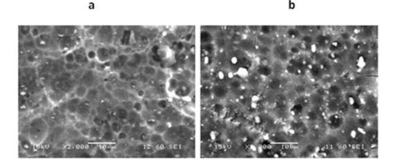
Fig. 8: SEM images of the surface of the conversion coating on the original (a) and modified (b) alloy
