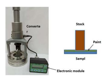
Fig. 1: Electronic adhesion meter PSO-MG4g
