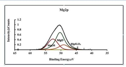
Fig. 4: XPS spectra of Mg2p in a modified inversion coating
