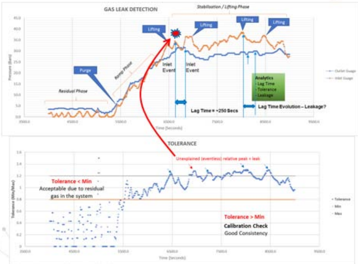
Figure 10: Lag time correction and leakage detection based on a tolerance window
