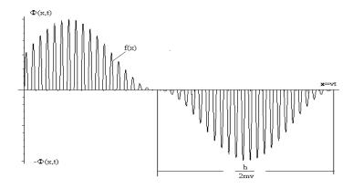
Figure 1: Behaviour of wave packet in linear dispersion medium
