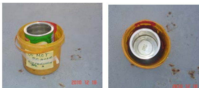
a. b. Figures 2 a. and b.: Photographs of improvised artificial pollen sampler
