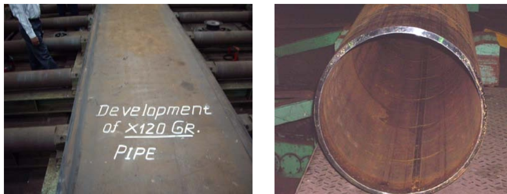
Figure 3 : Experimental X-120M Plate and Mechanically Expanded Line Pipe
