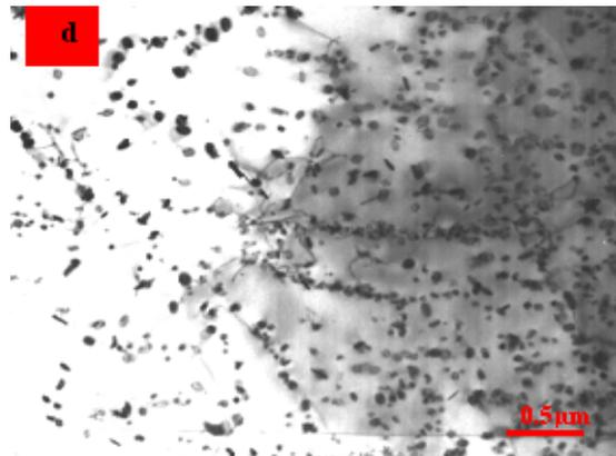
Fig.1 : Transmission electron micrographs showing the development of the microstructure during ramp heating at 100°C h-1 to (a) 300°C, (b) 350°C, (c) 400°C and (d) 550°C
