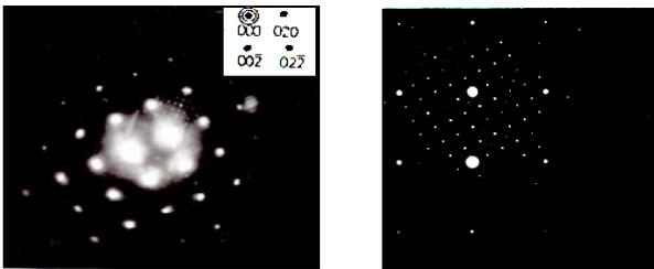
Fig.2 : Selected area diffraction pattern (SADP) from a dispersoid particles of type  $Al_{15}(Fe, Mn)_3Si_2$  phase
