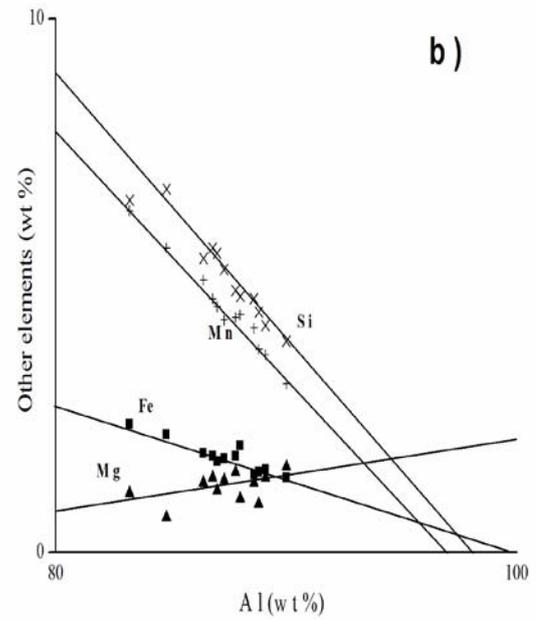
*Fig.4 :* Chemical composition data of the dispersoid particles in alloy II water quenched after ageing for
