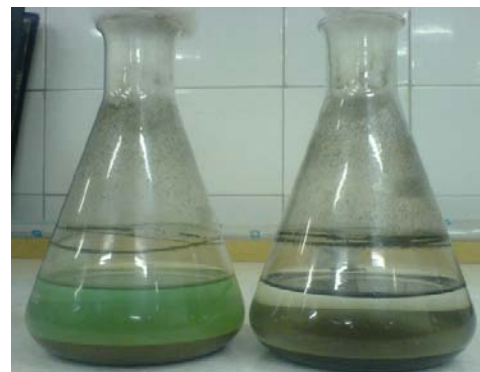
Figure 6: Color change due to bacterial activity and extraction of Cu in medium.
