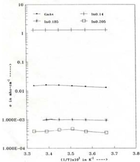
Figure 3.1 : Variation of conductivity with temperature of  $\text{In}_x\text{Ga}_{1-x}\text{As}$
