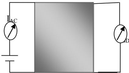
Figure 2.2 : Circuit for Hall Effect Measurement
