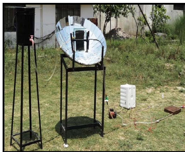
Fig 4.4 : Latent Heat Storage Solar Cooking Unit
