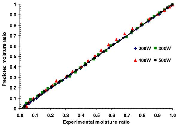
Figure 2 : Comparison of experimental moisture ratio with predicted moisture ratio from the Midilli model for carrot slices
