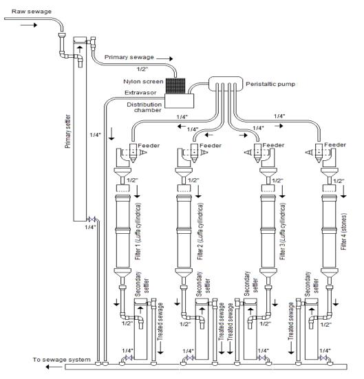
*Figure 4 :* General arrangement of the pilot plant, consisting of a primary settler, and four parallel and identical secondary biologic systems, three of them operating with *Luffa cyllindrica* as biofilm support medium (F1, F2, F3), and the last one using stones (filter 4).
