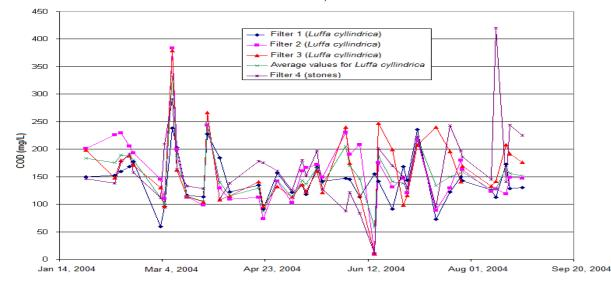
*Figure 10*: Chemical oxygen demand (COD) downstream the trickling filters filled with *Luffa cyllindrica* and downstream the filter filled with stones (downstream the secondary settlers): temporal series.
