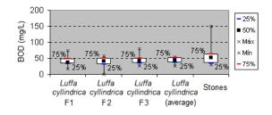
*Figure 9*: Box-whisker graphics for biochemical oxygen demand (BOD<sub>5,20</sub>) downstream the filters filled with *Luffa cyllindrica* (F1, F2, F3 and average value) and downstream the filter filled with stones (downstream the secondary) settlers
