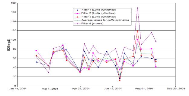
*Figure 6*: Biochemical oxygen demand (BOD<sub>5</sub>, <sub>20</sub>) downstream the trickling filters filled with *Luffa cyllindrica* (F1, F2, F3 and average value) and downstream the filter filled with stones (upstream the secondary settlers): temporal series.
