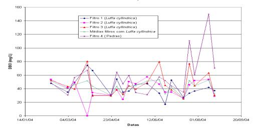
*Figure 8*: Biochemical oxygen demand (BOD<sub>5</sub>, <sub>20</sub>) downstream the trickling filters filled with *Luffa cyllindrica* (F1, F2, F3 and average value) and downstream the filter filled with stones (downstream the secondary settlers): temporal series.
