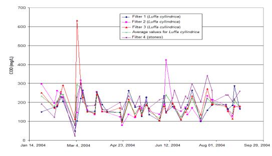
*Figure 8*: Chemical oxygen demand (COD) downstream the trickling filters filled with *Luffa cyllindrica* and downstream the filter filled with stones (upstream the secondary settlers): temporal series.
