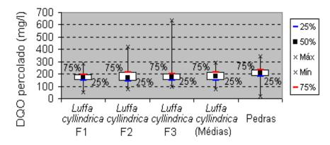
*Figure 9 :* Box-whisker graphics for chemical oxygen demand (COD) downstream the filters filled with *Luffa cyllindrica* (F1, F2, F3 and average value) and downstream the filter filled with stones (upstream the secondary settlers).
