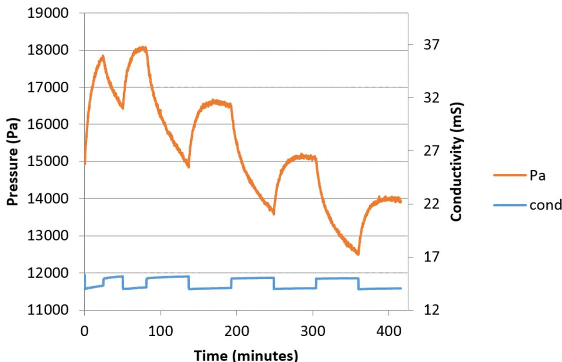
*Figure 1.6* : An ionic strength test immediately after synthesis where the initial test was conducted within 1 week of the hydrogel synthesis. The hydrogel was tested for 5 continuous cycles. After the first 2 cycles, the continuous system was modified in order to allow the swelling and deswelling to come to an equilibrium point
