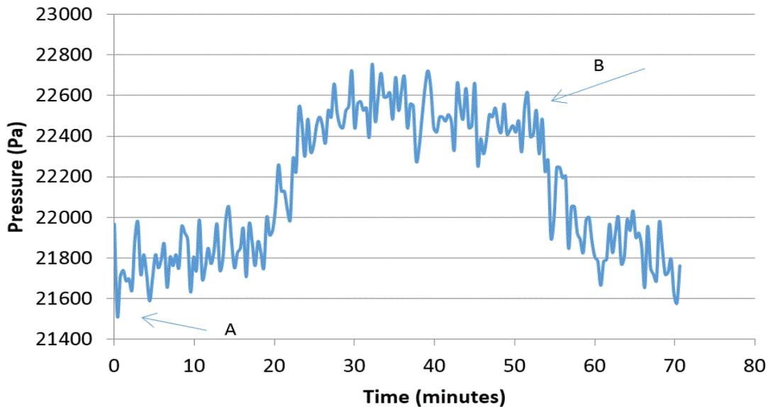
*Figure 1.3:* An ionic strength test after 18 months where the average first order response time was 9 minutes for swelling and 8 minutes for deswelling. The average magnitude response change was 1.1 KPa for swelling and 1.6 KPa for deswelling
