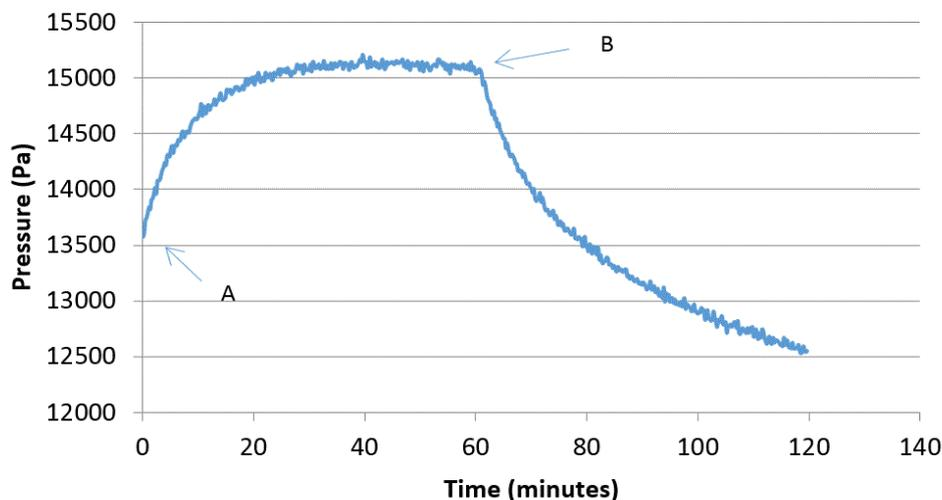
**Figure 1.1 :** An ionic strength test where the ionic strength concentration was decreased (from 165 mM to 155 mM) at point A. When the hydrogel sample came to equilibrium, the concentration was changed to a higher concentration at point B (from 155 mM to 165 mM). The average first order response time was 22 minutes for swelling and 17 minutes for deswelling. The average magnitude response change was 1.6 KPa for swelling and 2.8 for deswelling
