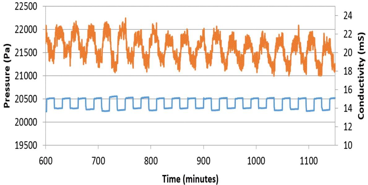
Figure 1.9 : A stable region of the 300 cycle test shows 18 cycles of the third test that illustrate the stability of the hydrogel swelling and deswelling
