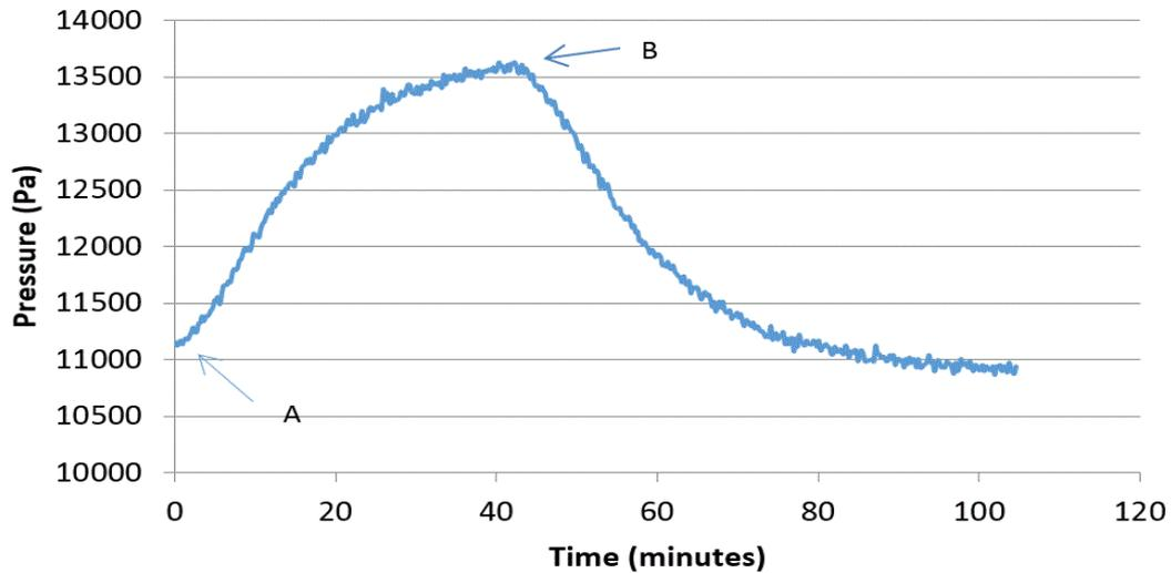
*Figure 1.2:* An ionic strength test after 9 months where the average first order response time was 9 minutes for swelling and 14 minutes for deswelling. The average magnitude response change was 2.4 KPa for swelling and 2.6 KPa for deswelling
