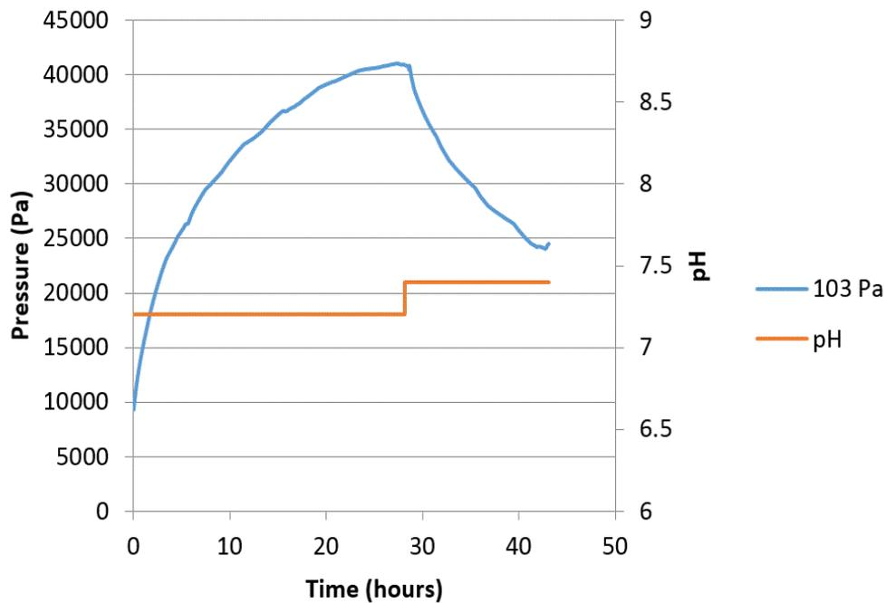
Figure 1.5: A pH response test from pH 7.2 to 7.4 of the hydrogel sample in the M-Biotech sensor after simulating travel conditions
