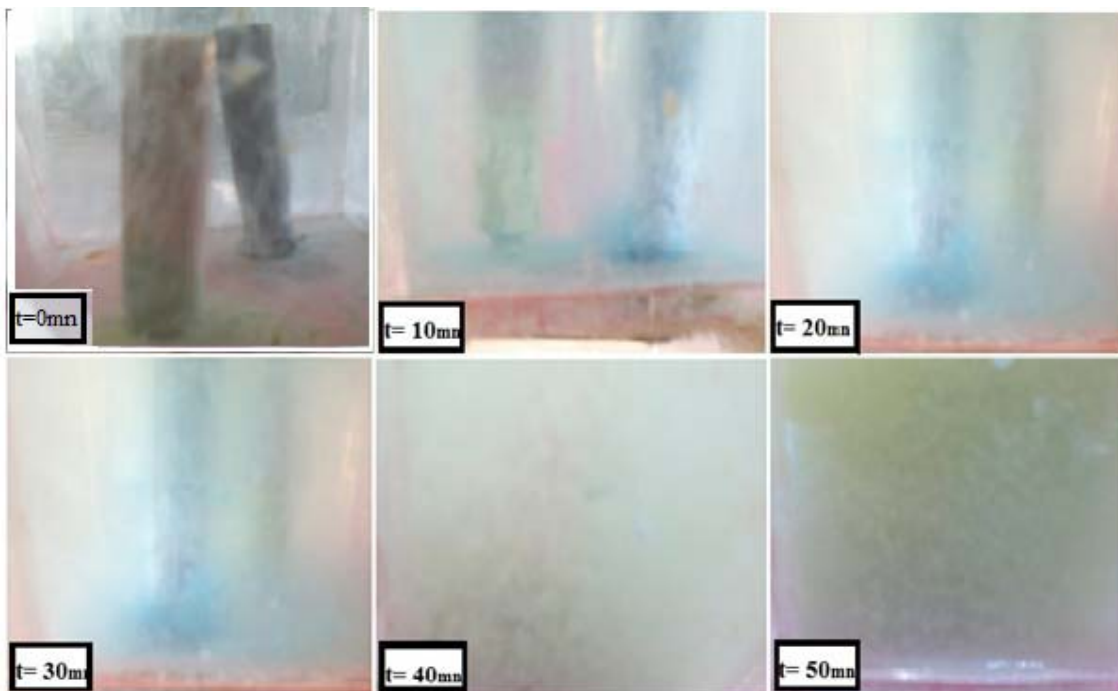
Figure 6 : Evolution of the corrosive condition of the electrodes
