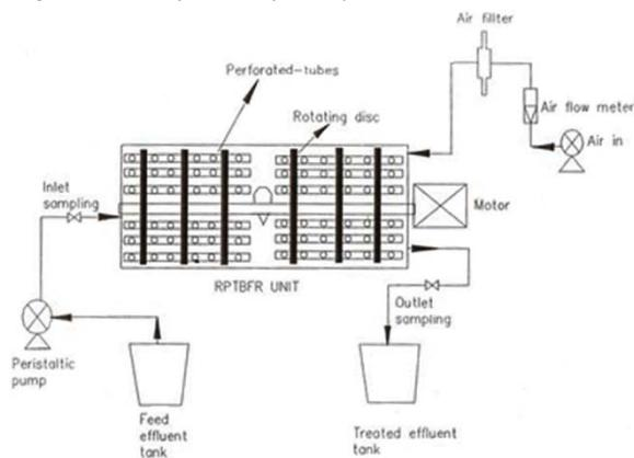
Figure 1 : Schematic diagram of rotating perforated tubes biofilm reactor
