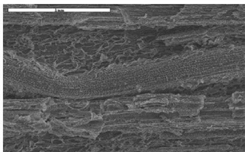
Fig. 5 (c) : Basel End DPF treated 0.75%NaOH
