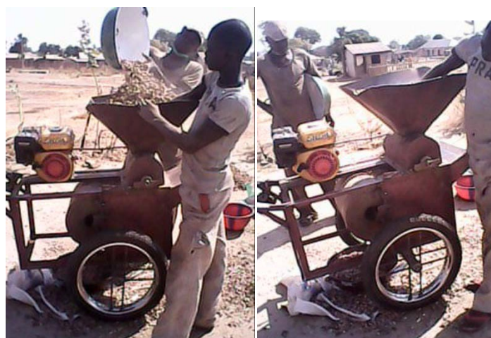
Figure 3 : Photo Type of a Multipurpose Post Harvest Machine for Shelling and Threshing Maize, Cowpea and Groundnut. It Was Introduced In 2009 Reduce Excess Post Harvest Losses in the Study Zone.
