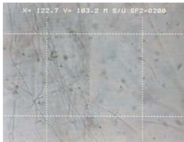
Figure 19 : Biomass found in stones media: bacteria Sphaerotilus natans .
