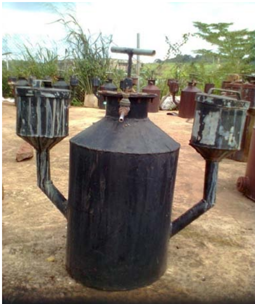
Figure 2 : Fixed-dome biogas digester (NCERD UNN)
