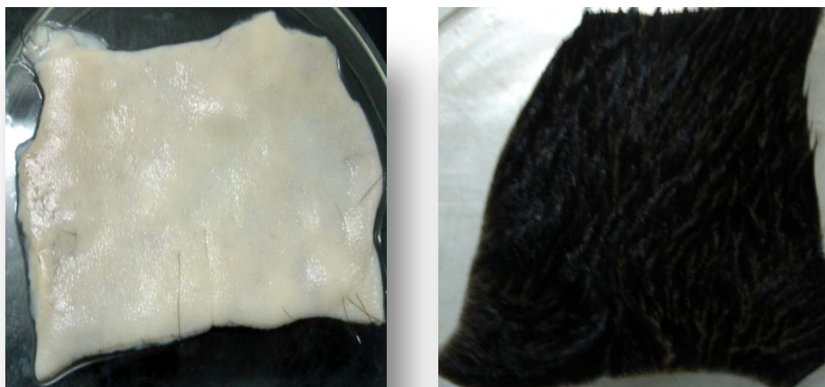
Figure 6 : Enzymatic dehairing by B. subtilis on left, control is on the right (without enzyme)
