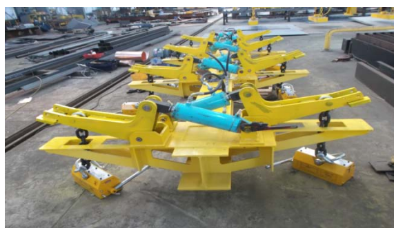
Fig. 12 : Image of a assembled hydraulic-magnetic clamp
