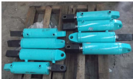
Fig. 10 : Image to show the hydraulic cylinder used for the hydraulic, magnetic clamp
