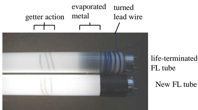
**Figure 33 :** Photograph that indicates getter action of periodically polarized phosphor particles under EEs that are operated with external AC driving circuit of  $3\text{ kV}_{\text{rms}}$  and 30 kHz
