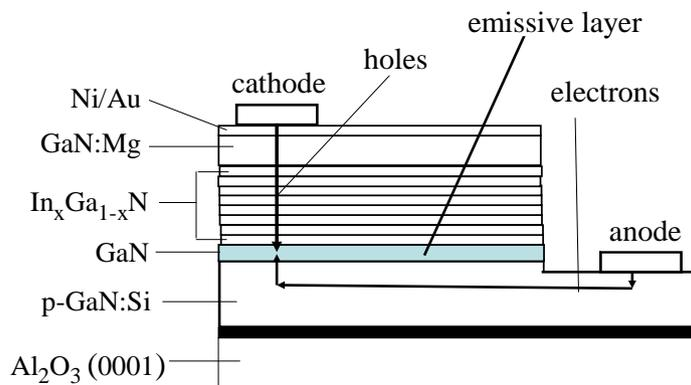
Figure 3 : Structure of LED lamp. Junction generates lights by recombination by EHs
