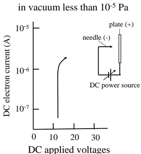
Figure 11 : Experimental curve of DC current between needle electrode and plate anode in vacuum at  $10^{-5}$  Pa
