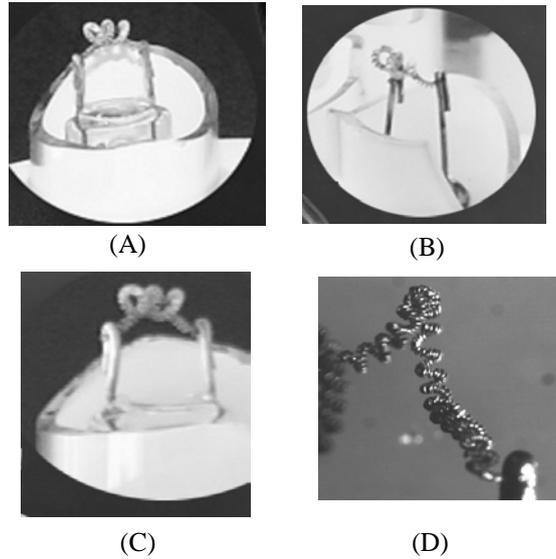
Figure 5 : Photographs of twisted W-filament coils with BaO particles in commercial FL tubes
