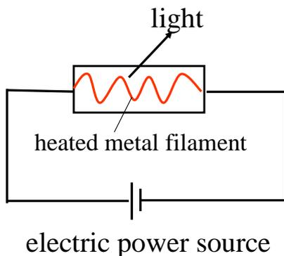
Figure 1 : Schematic explanation of metal filament lamp
