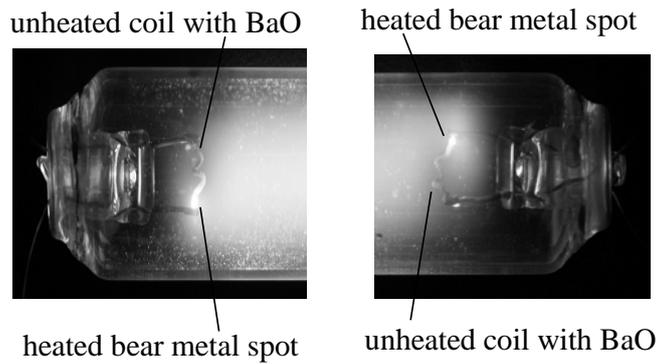
Figure 6 : Photographs of working W-filament coil with BaO particles in lighted FL tube
