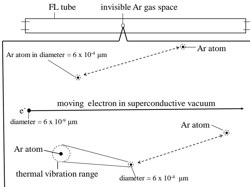
**Figure 16 :** Schematic explanation of superconductive vacuum between Ar atoms for moving electrons from needle cathode to anode in lighted glass tube. Moving electrons do not have electric resistance by thermal perturbation of neighboring Ar atoms
