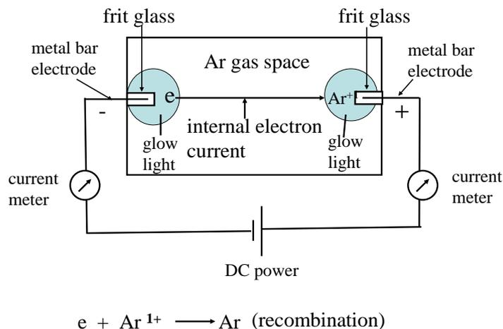
Figure 21 : Explanation of moving electrons between volumes of glow light as cathode and anode of internal DC electric power generator formed in Ar gas space
