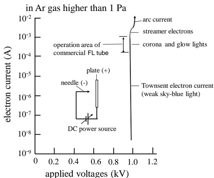
Figure 15 : Experimental curve of DC current between needle electrode and plat anode in Ar gas pressures at 10 Pa
