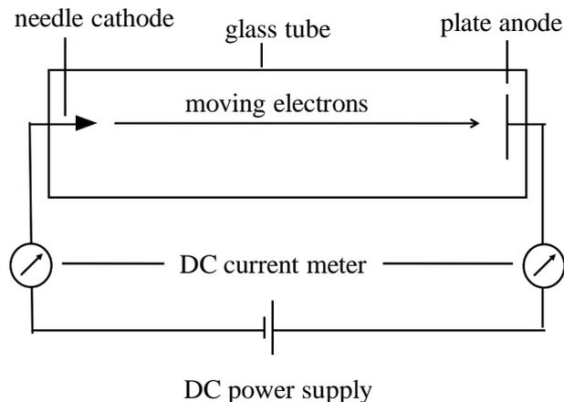
Figure 10 : Explanation of structure of experimental glass tube for electron emission from needle cathode and plate anode under DC power supply
