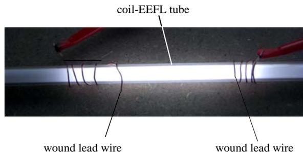
Figure 25 : Photograph of prototype of lighted coil-EEFL tube under 2 kV of DC driving circuit
