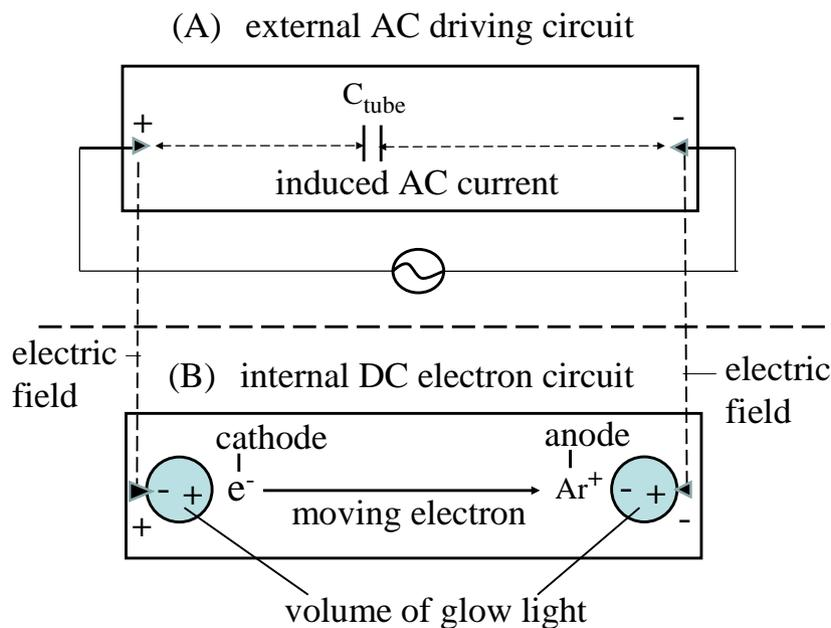
Figure 22 : Schematic explanation of electric closeness of AC driving circuit by AC induced current from  $C_{tube}$  (A) and moving electrons from cathode to anode of internal DC electric power generator that is formed in Ar gas space without electron flow from external AC driving circuit (B)
