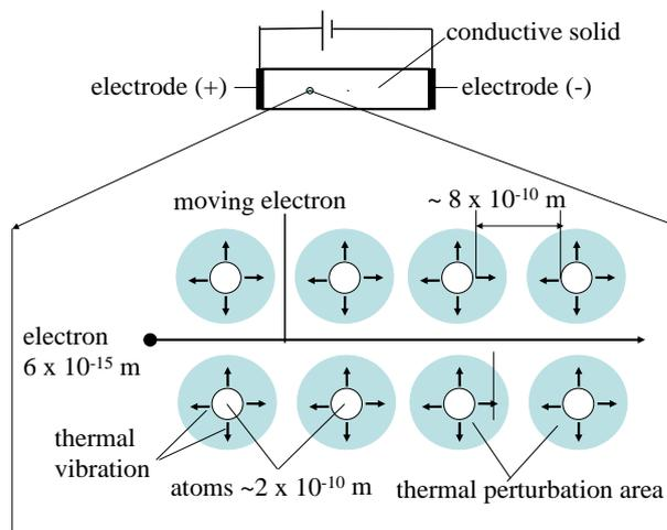
Figure 2 : Schematic illustration of moving electron in narrow vacuum space between atoms at lattice sites in semiconductor crystal
