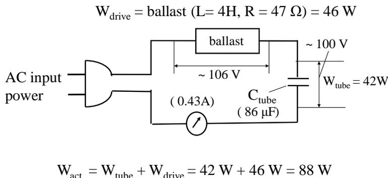
Figure 9 : Schematic explanations of AC driving circuit of FL tube and AC power consumptions of  $W_{\text{act}}$  that is composed with  $W_{\text{drive}}$  at ballast and  $W_{\text{tube}}$  at FL tube
