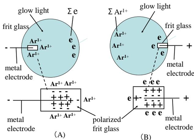
Figure 20 : Formation mechanisms of volume of glow lights on polarized frit glass layers that cover on needle cathode (A) and needle anode (B)
