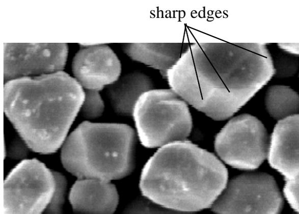
Figure 24 : Photograph of SEM (x 3000) of ideal phosphor particles having sharp edge-lines and points for phosphor screen in coil-EEFL tube
