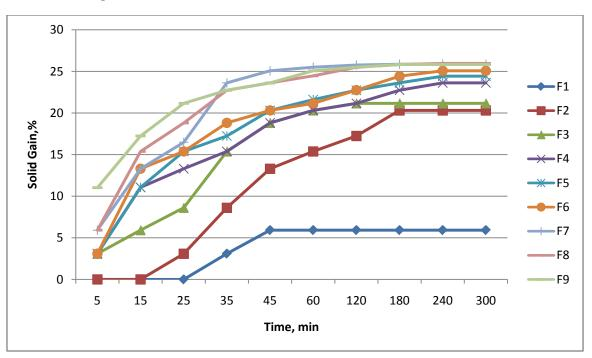
Figure 3 : Effect of NaCl concentration and immersion time on Solid Gain
