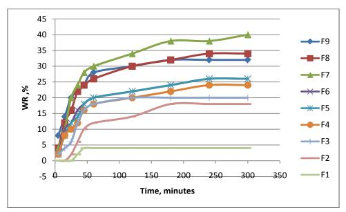
Figure 1 : Response of weight reduction WR (%) to solute concentration and immersion time
