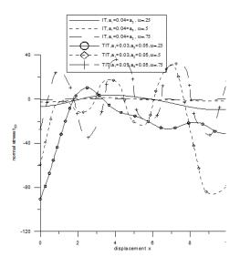
Figure 2 : Variation of Normal Stress t<sub>33</sub> with Distance X(Concentrated Force)
