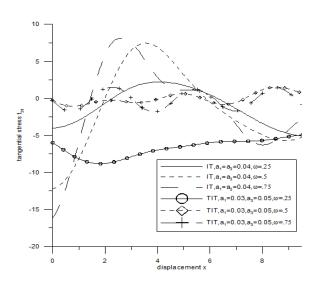
Figure 11 : Variation of Tangential Stress t<sub>31</sub> with Distance X(Concentrated Thermal Source)
