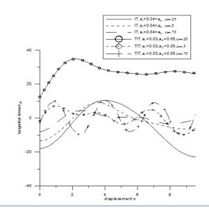
Figure 3 : Variation of Tangential Stress t<sub>31</sub> with Distance X(Concentrated Force)
