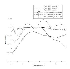
Figure 6 : Variation of Normal Stress t<sub>33</sub> with Distance X(Uniformly Distributed Force)
