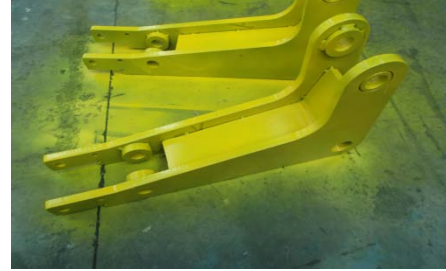
Fig. 11 : Image of magnetic arm unit composed of 2 side plates and 1 rib plate to connect the hydraulic cylinders
