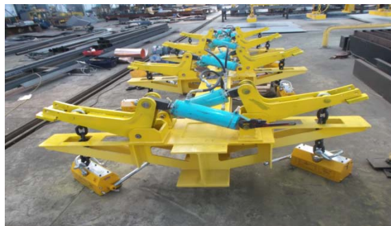
Fig. 12 : Image of a assembled hydraulic-magnetic clamp
