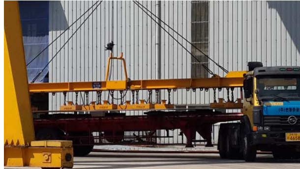
Fig. 2 : Actual view of current magnetic crane device
