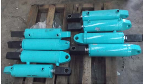
Fig. 10 : Image to show the hydraulic cylinder used for the hydraulic, magnetic clamp
