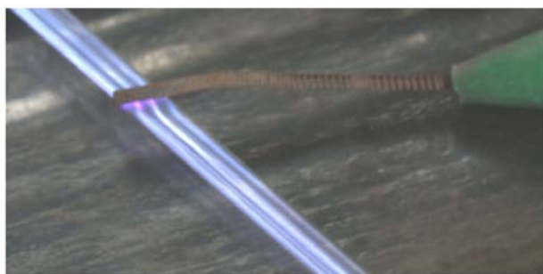
Figure 34 : Photograph of lighted vacuum-sealed glass tube under Tesla coil. Tubes are immediately after vacuum seal from pumping facility
