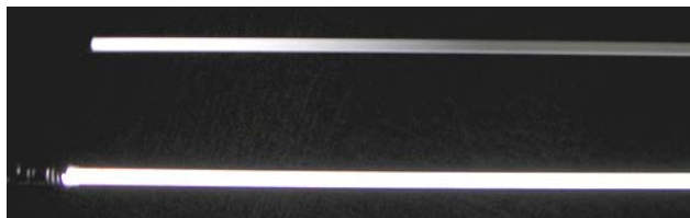
Figure 32 : Photograph of lighted coil-EEFL tubes; with commercial phosphor screen (above) and the improved phosphor screen (below)
