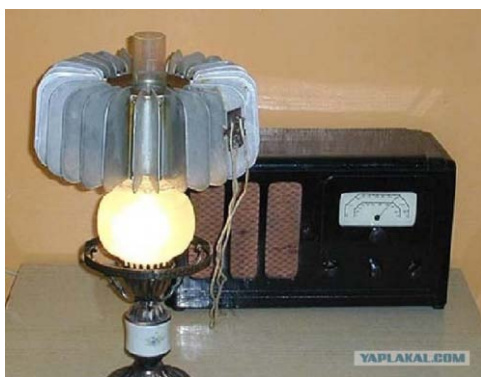
Fig. 3 : Charge distribution in the flame of a kerosene lamp can be used to obtain the electric current required to function the radio receiver.
