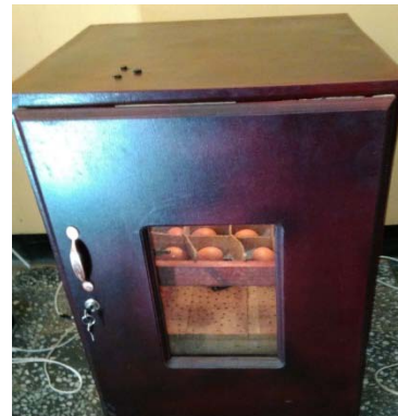
Figure 11 : The prototype microcontroller base egg incubator used in this study
