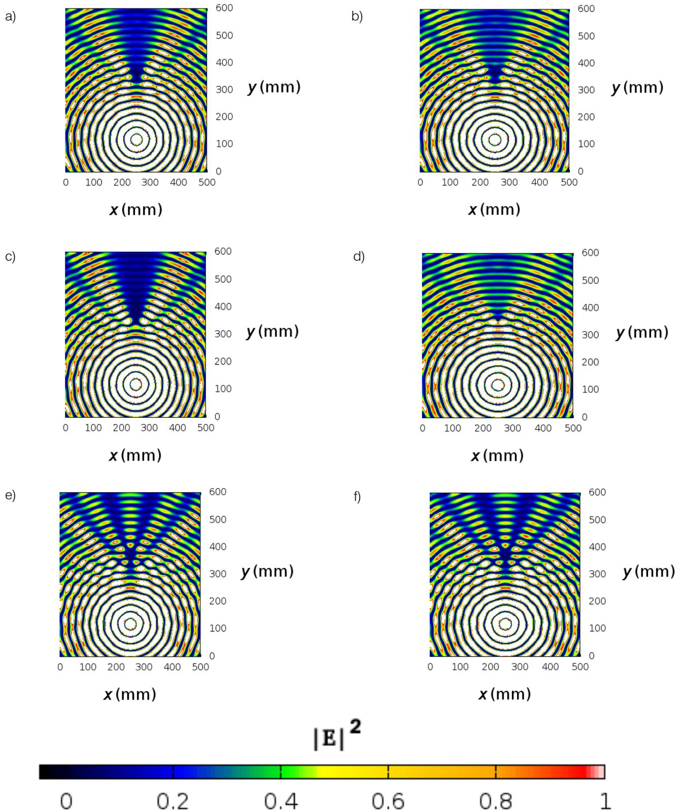
Fig. 6: Power propagation in FDTD at fixed time. In (a, c, e) plasma gradient is include and (b, d, f) only the metamaterial is keep for the result, (a & b)  $\mu_r = \mu_\theta = 0.268$ ; (c & d)  $\mu_r = \mu_\theta = 1$ ; (e & f)  $\mu_r = 1$  and  $\mu_\theta = 0.268$
