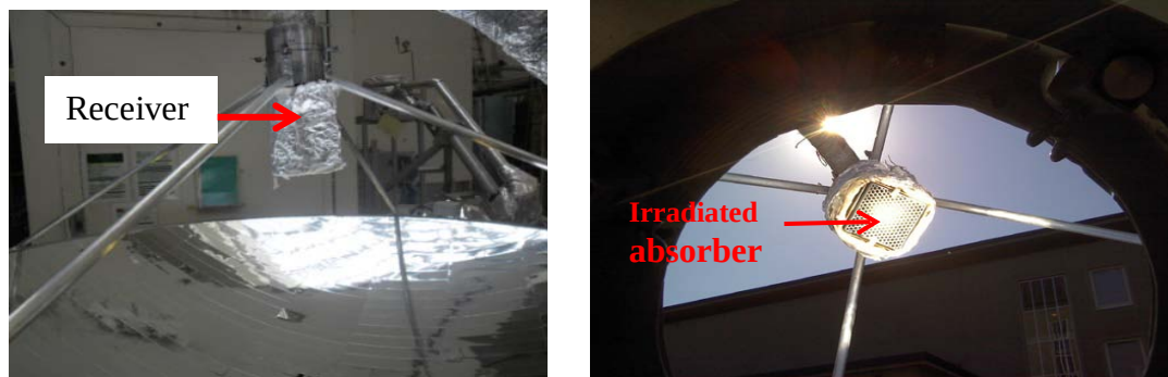
Figure 2: Shows receiver mounted on the setup (left) and irradiated receiver during tests (right)
