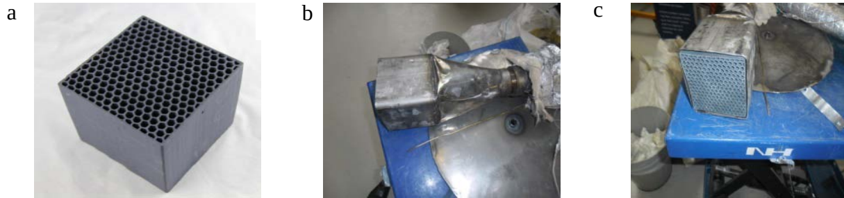
Figure 1: Showing a) SiC honeycomb absorber, b) Absorber housing and c) The receiver
