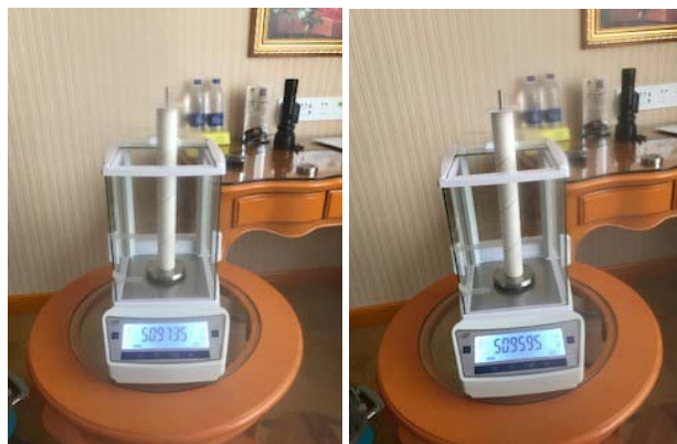
Figure 1: A long paper tube is put on the surface of electronic scale to make the influence of the magnet to the scale negligible.
