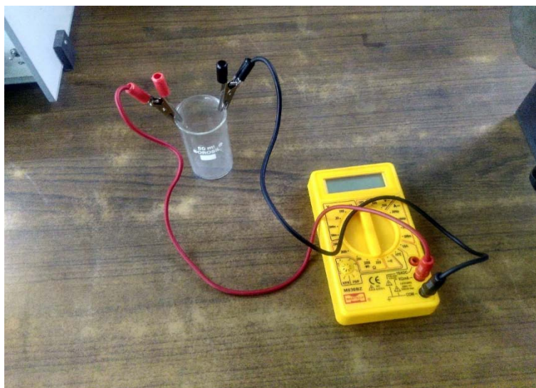
Fig. 4: Conductivity measurement arrangement
