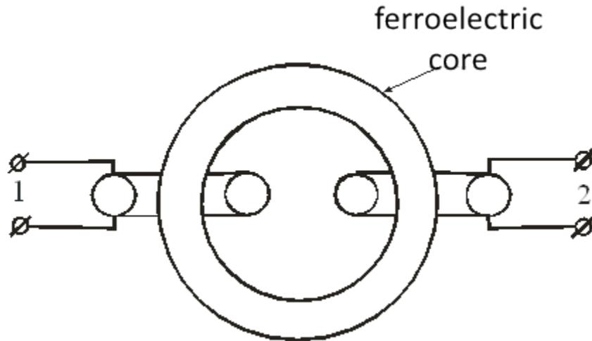
*Fig. 2:* Transformer with the toroidal ferroelectric core
