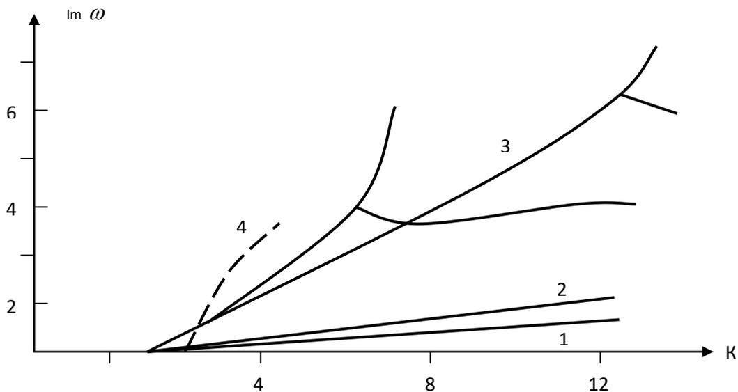
*Figure 4:* Dependence of the imaginary part of the complex frequencies ( $\text{Im}$ ) to wave numbers ( $k$ ) for different values of  $\eta$ : 1-0.0009; 2-0.0018; 3-0.18; 4-0.19;--- by the formula (22)
