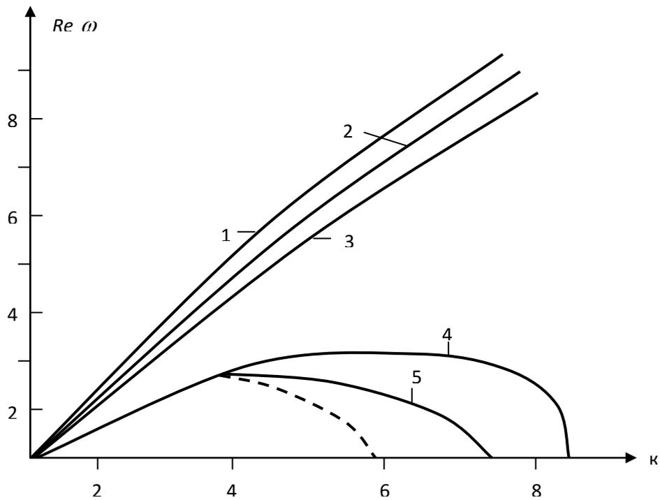
*Figure 1:* Dependence of the real part of the complex frequencies ( $\text{Re } \omega$ ) to wave numbers ( $k$ ) for different values of  $\eta$ . 1-0.0009; 2-0.0018; 3-0.18, 4-0.19, 5-according to the formula (20); By the formula (22)
