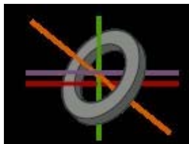
Fig. 1: Diagram of the functioning of memory element on the ferrite core
