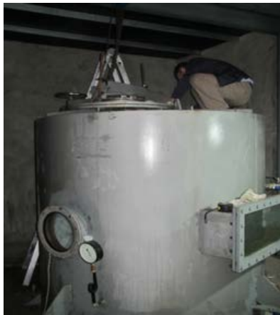
Fig.6: Vacuum tank with a torsion scale placed in
