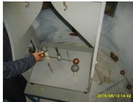
Fig.7: A homemade Cavendish torsion scale placed in the vacuum tank
