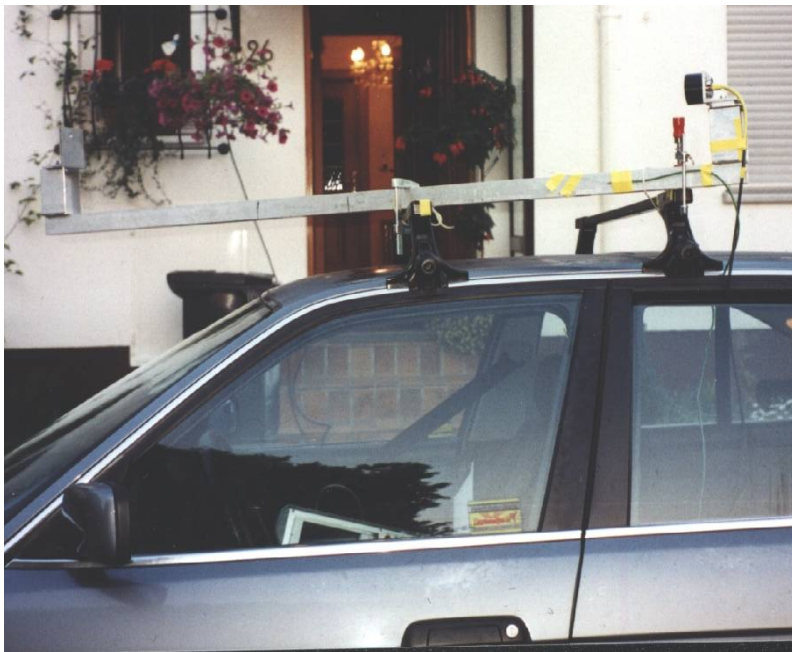
Fig. 9: Photo showing the Measuring Gauge Mounted on the Car's Top in 2000
