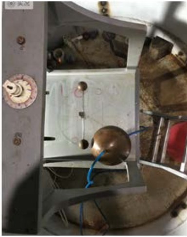
Fig. 11: Top view of gravity balance in the vacuum tank
