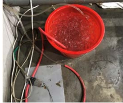
Fig.12: A small pump and a bucket used to fill in the large hollow copper ball with hot or icy water
