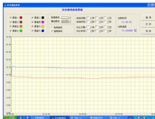
Fig. 17: The temperature curve of the big copper ball and the small copper ball over time. The blue line
