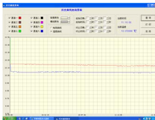
Fig. 16: The temperature curve of the big copper ball and the small copper ball over time. The red line represents the temperature of the big copper ball, and the blue line represents the small copper ball
