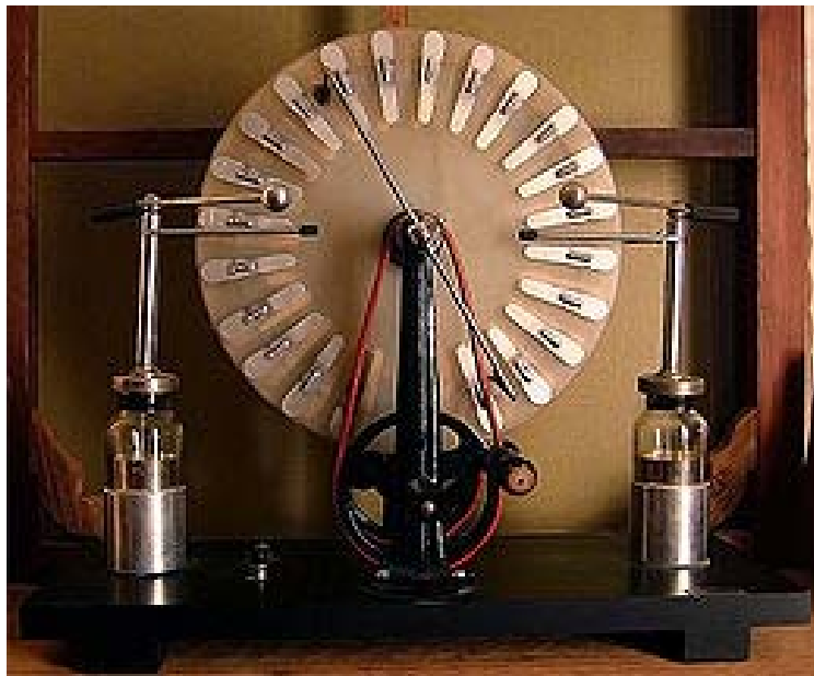
Fig. 2: The electric generator, invented by James by Whimshurst
