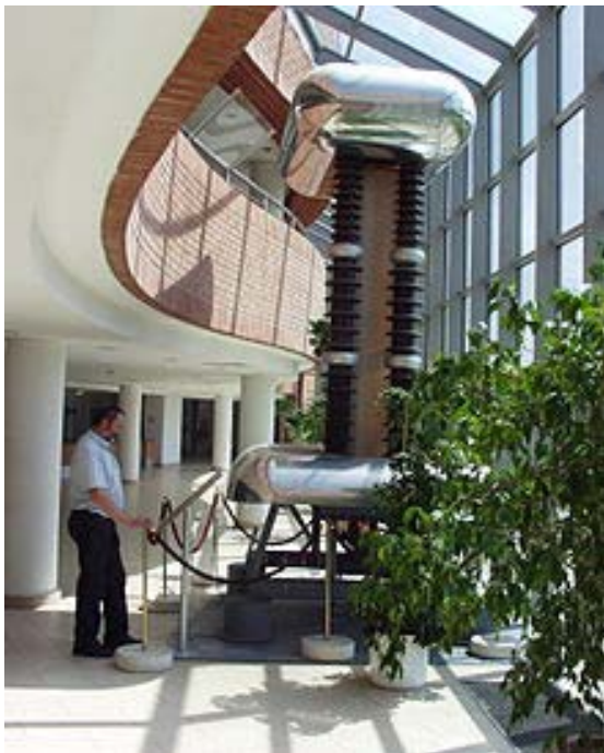
Fig. 3: Belt generator for the first in Hungary linear accelerator
