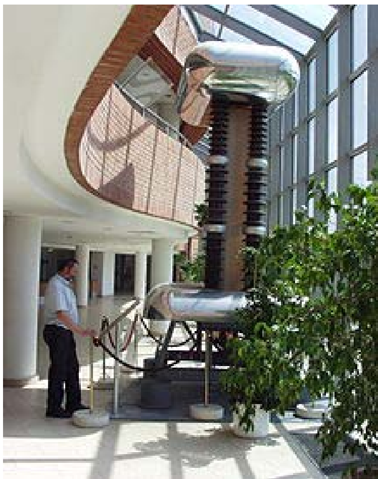
Fig. 3: Belt generator for the first in Hungary the linear accelerator, on which in 1952 the year stress MV was 1 obtained
