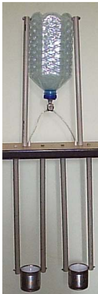
Рис. 10: General view of the experimental layout of the Mende electrostatic generator
